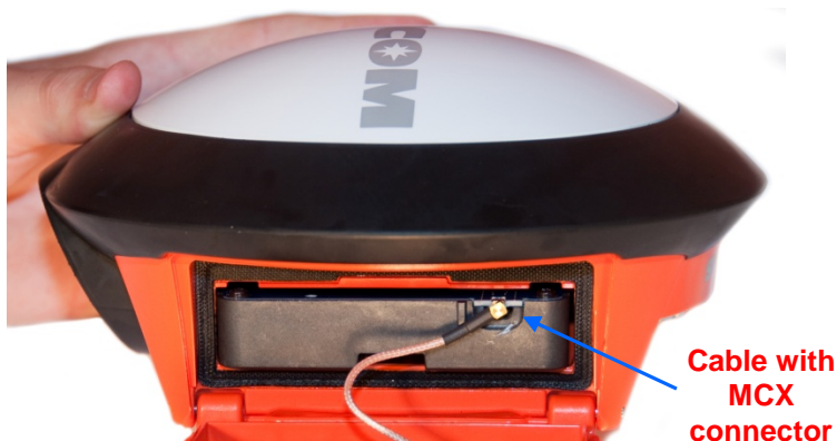
Figure 58: Radio Modem Installed in SF-3040
