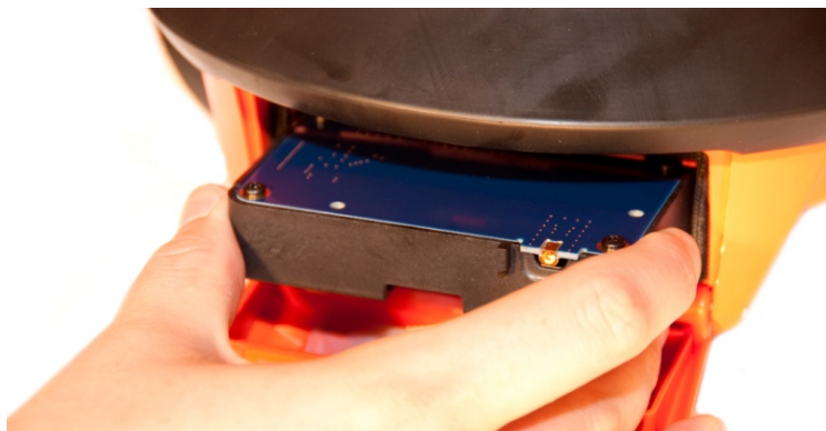
Figure 57: Radio Modem Installation
