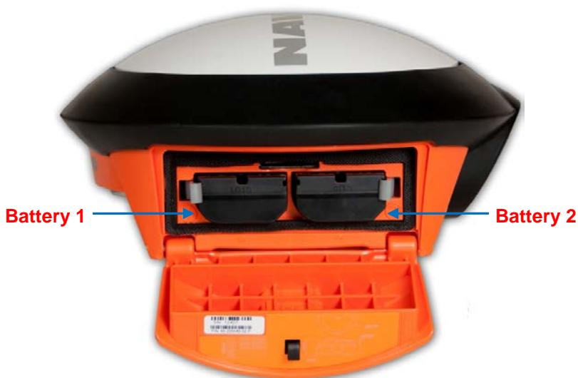
Figure 54: SF-3040 Battery Packs Installed in Battery Chamber
